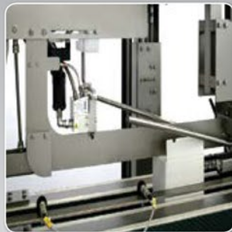
Automatic box closing machine with closing of the upper flaps by means of Hot Melt glue
