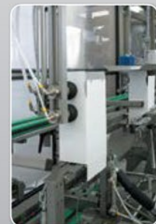
Automatic box erector with closing of the lower flaps by means of Hot Melt glue
