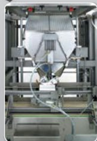
Automatic bag filler complete with box introduction system
