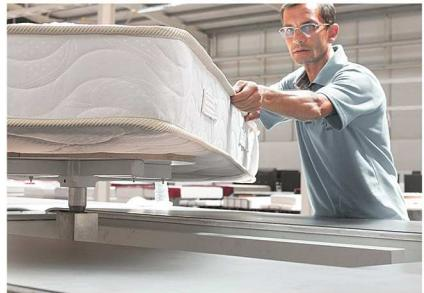
**Quality Control and Cleaning Conveyor:** The machine is designed to help the operators to do the cleaning and control the quality of the mattresses coming from the line. With the help of Pedals the mattresses can be turned 360° and flip flopped.
