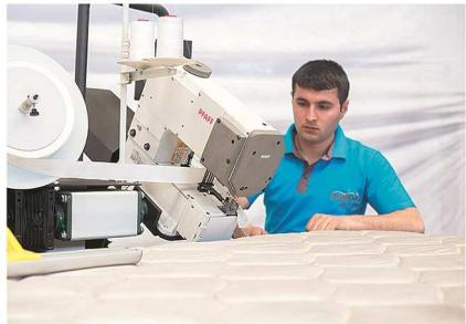
**Automatic Tape Edge Machine:** This machine is designed to close the edges of the mattresses from 5cm to 40cm high easily with the help of the Mattress Turning Arm. Thanks to the Automatic Flip Flopping arms the machine can sew the both sides of the mattresses if needed.
