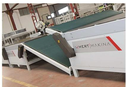
**Mattress Flip Flopping Conveyor:** Flipping the mattresses other side to be sewed on the next machine thanks to its high trapeze belt system.
