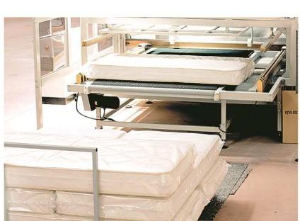
**Automatic Mattress Packaging:** Packing (wrapping) the mattresses with automatic dimension detection and automatic pressing (vacuuming) system.
