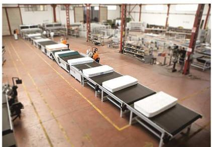
**Shape of Line:** Line is transformed straight - «L» or «U» form by diving with additional conveyors according to requested capacity and free space.
