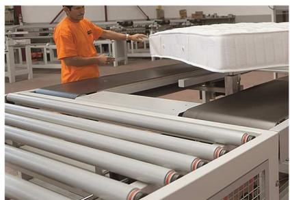
**Cross Conveyor:** This conveyor is directing carcass, mattresses, to different directions according to the shape of line «L», «T», «U»
