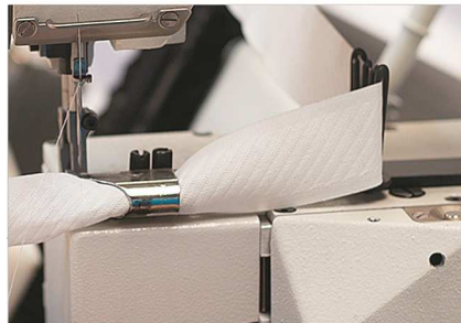
Needle Position; Automatic needle and foot lifting with pneumatic system.
