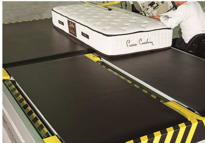
Flip - Flopping Mattresses; Dynamic Mattress Positioning systems and eliminating operator handling.
