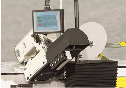
Speed adjustment; speed adjustment on screen for straight sewing and corner sewing speed
