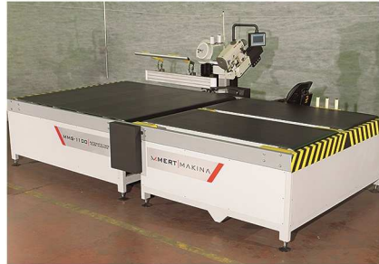
Conveyor System; anti-static PVC belt
