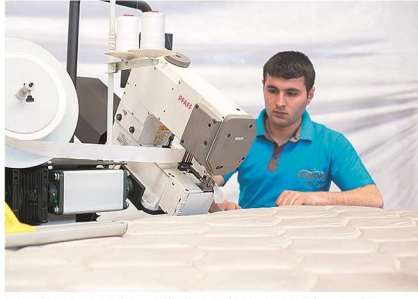
Sewing Machine; Chain Stitch machine with double transport for thick materials and non-stop stitching.
