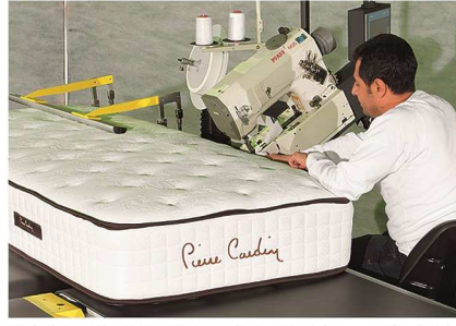
Height Adjustment; Sewing machine angle and up down adjustment for able to work on mattress with different dimension.
