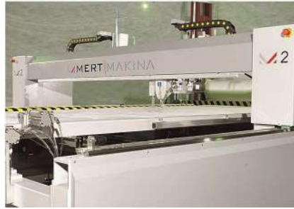
Automatic "Parking Position" when top and bottom thread breaks and ends Alt ip ve üst ip kopma / bitiminde otomatik park pozisyonu
