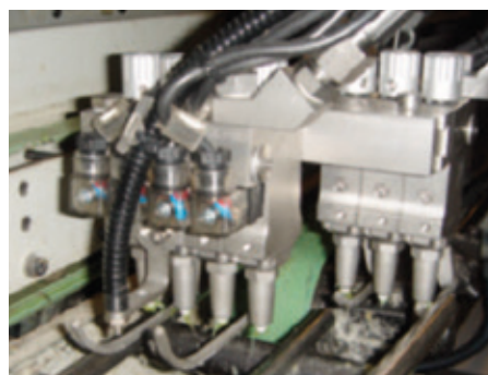
Modular GTE-13/M: 4 glue distributors installed on one block in the front and 3 on the back, connected by a moving rail to set distance between glue nozzles.
